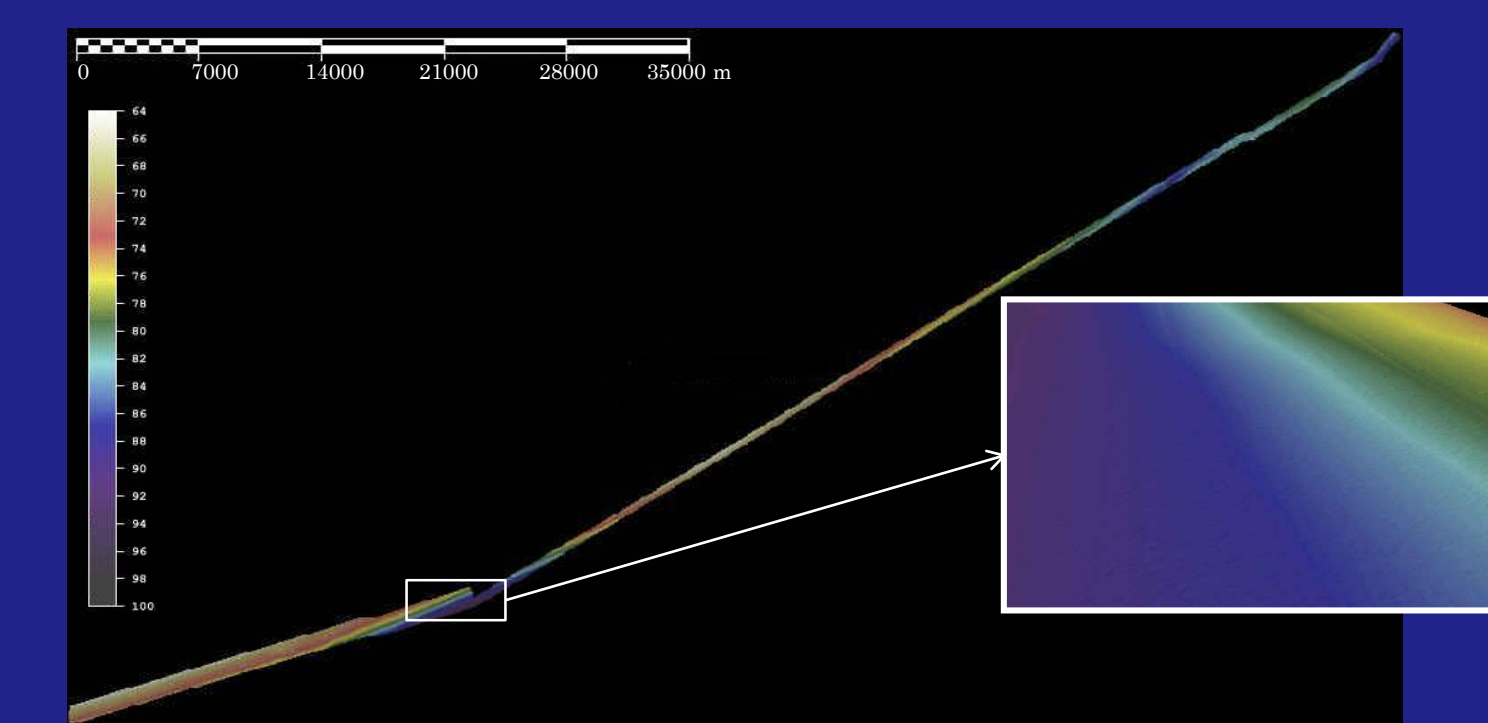
Figure 4. 2-D bathymetric image southeast of Vaca Key with depths ranging between 64.5 and 98 m. Note the gently sloping, featureless surface of the 3-D image (inset) at 2.5x vertical exaggeration.
